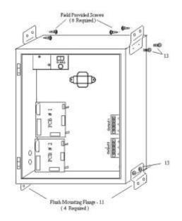
For best Flush Mounting results, recess face of enclosure's lip  $\frac{1}{2}$ " behind wall finish
