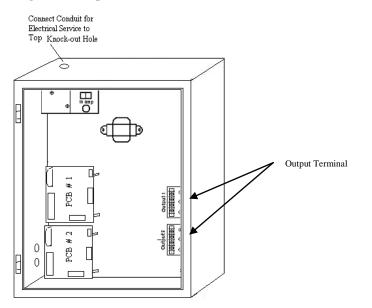
**NOTE:** This Unit is provided with an Output Terminal per pcb as shown in Figure 6.
