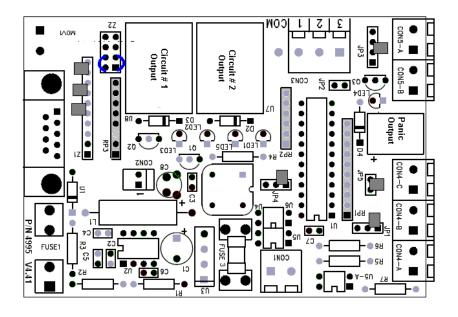
When V4.41 two circuit pcb is included in the Shop Controller unit, the figure above reflects the typical arrangement and configuration for this board. However, in some cases where 120 vac outputs are required for the unit, then the configuration of the board will be slightly different.
